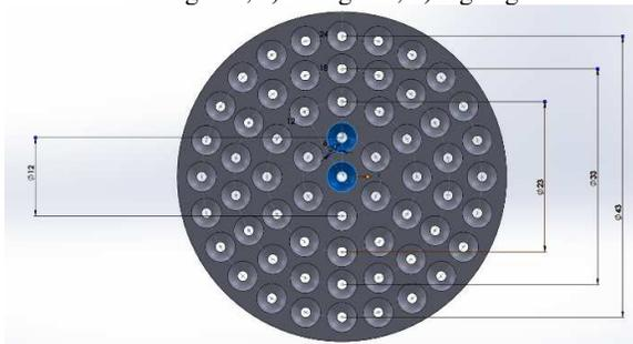
**Fig.4.** Arrangement of holes at the surface
