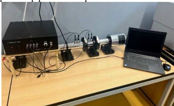
**Fig.1.** Impedance tube HO-ED-A-03 type
