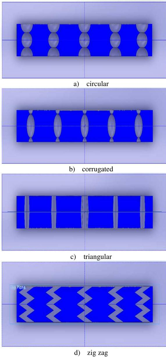
**Fig.3.** The new geometry of holes: a) circular; b) corrugated; c) triangular; d) zig zag
