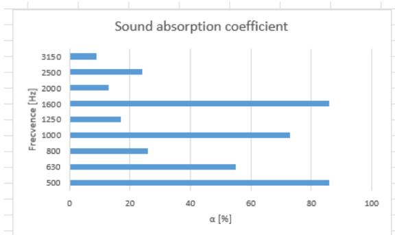
Fig.8. Sound absorption properties at each frequency.
