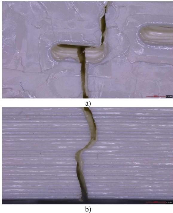
**Fig.10.** Surface micrograph: a) on the surface; b) on the height
