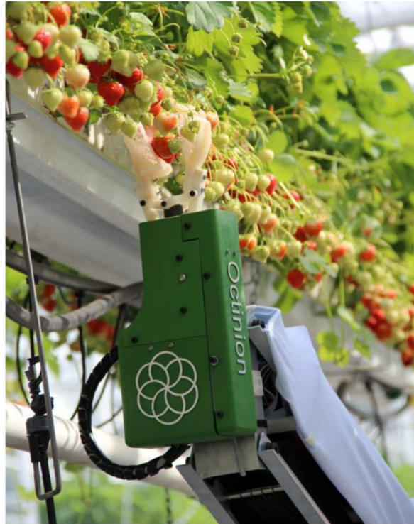
Fig. 1. Octinion Strawberry Picker Robot [26]
