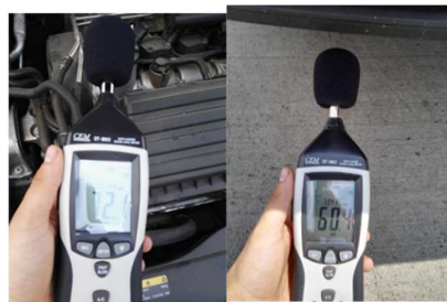
Fig. 8. Steady-state meters (from engine compartment, i.e. from exhaust pipe)
