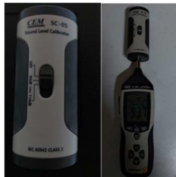
Fig. 2. Sound level meter calibrator and calibration operation
