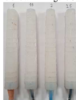
Fig. 5. Final version of the 4 actuators with different wall thicknesses.
