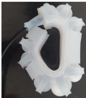
Fig. 6. 1.5 mm wall thickness multi-segment actuator pressurized to 100 kPa.
