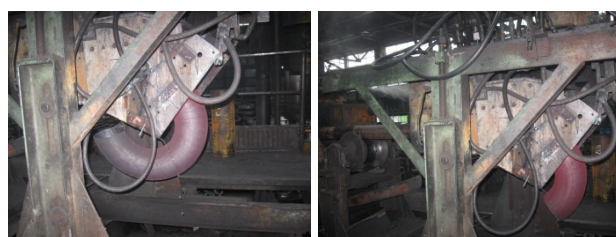
Fig. 4. Bend manufacturing by mandrel pulling and induction heating ( D_n 168.3 x 4.5 mm)
