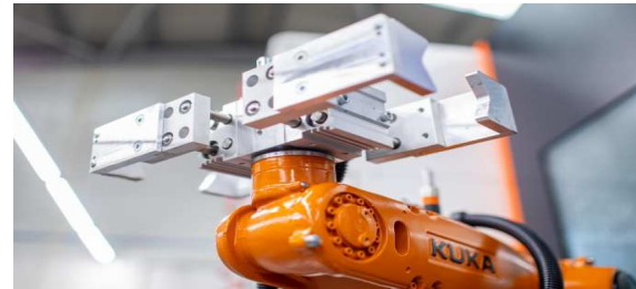
Fig.7. The robot gripper feeding the CNC [7]
