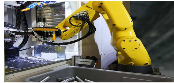
Fig.6. CNC feeding with robot equipped with 2 pairs of jaws [6]
