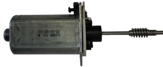
Fig. 3. Worm shaft from the construction of the seat adjustment mechanism of Mercedes car [6], [8].
