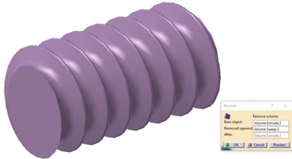
Fig. 9. 3D modeling of the helical profile of the worm shaft from the construction of the seat adjustment mechanism of an Audi car.
