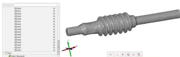
Fig. 23. The number of scans for the worm shaft from the construction of the seat adjustment mechanism of a Mercedes car.
