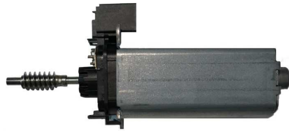
Fig. 2. Worm shaft from the construction of the seat adjustment mechanism of an Audi car [6], [8].
