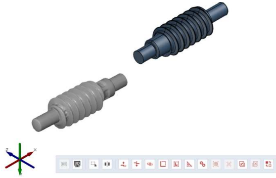
Fig. 26. Importing the scanned model and CAD model of the worm shaft from the construction of the seat adjustment mechanism of an Audi car.
