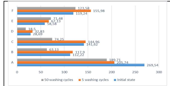
Fig. 2 Distribution of air permeability values under wet condition, after conditioning at 23° C and 85% humidity
