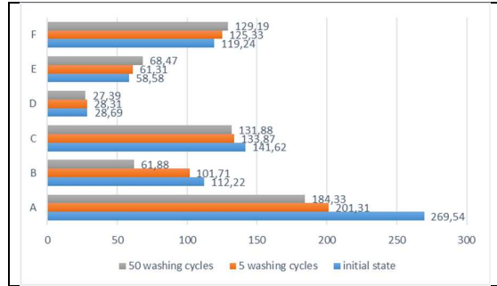
Fig. 6 Distribution of air permeability values prewash treatment, 7h of conditioning in saline solution and 3h of conditioning at -10^{\circ}\text{C}
