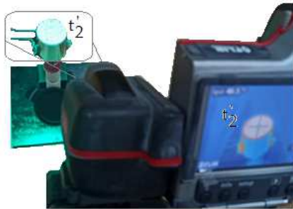
Fig. 12. Real – time monitoring of calcium silicate plate with T400 thermal imaging camera.
