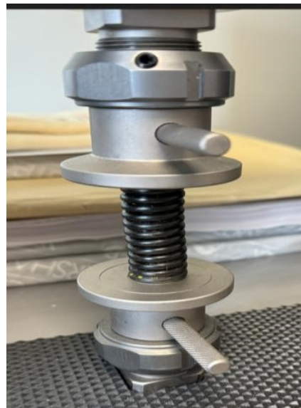
Fig. 2. Firing pin spring subjected to compression load
