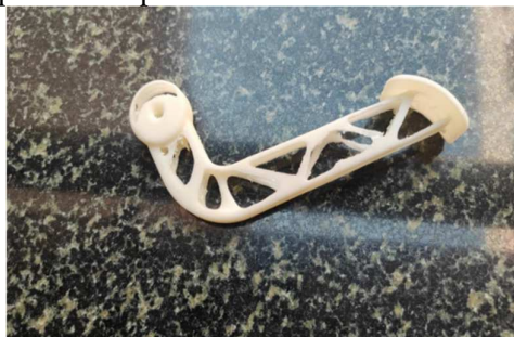
Figure 11: Prototype AM throttle pedal part made of ABS
