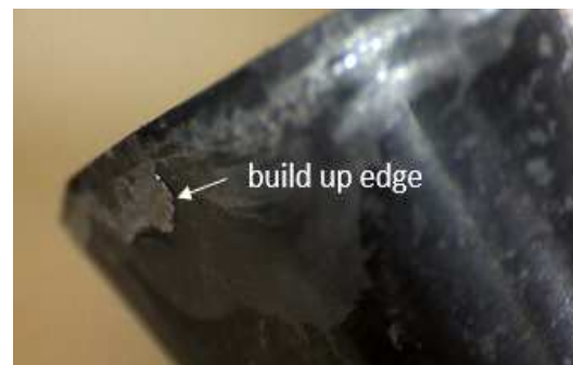
Fig. 19. Wear after 338 minutes machined and build up edge
