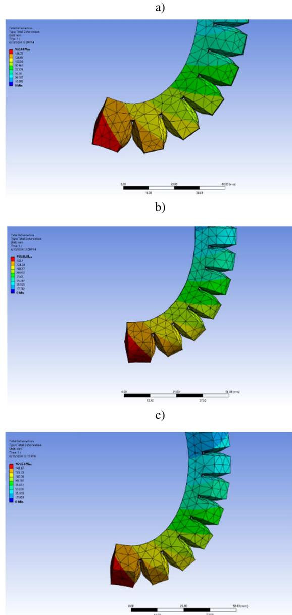
Fig. 10. Interaction between channels: a) actuator with a rectangular cross-section, b) actuator with a semi-circular cross-section, c) actuator with a triangular cross-section
