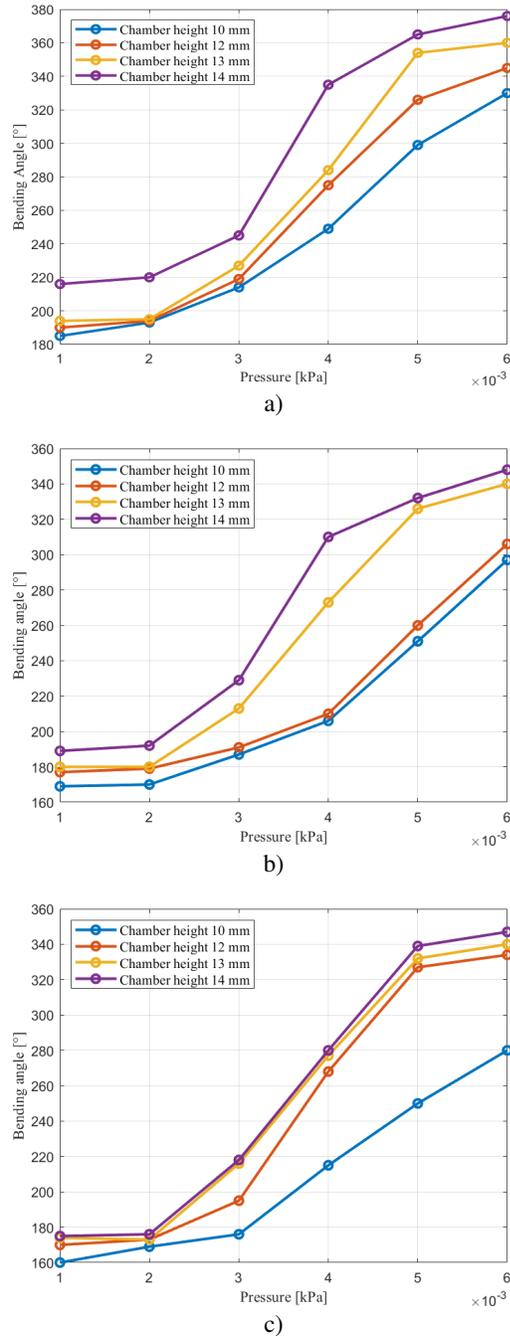
**Fig. 7.** The effect of pneumatic chamber height for: a) the actuator with a rectangular cross-section, b) the actuator with a semi-circular cross-section, c) the actuator with a triangular cross-section.
