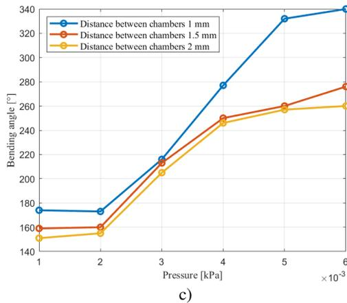
**Fig. 6.** The effect of pneumatic chamber spacing for: a) the actuator with a rectangular cross-section, b) the actuator with a semi-circular cross-section, c) the actuator with a triangular cross-section.
