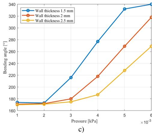
**Fig. 5.** The effect of pneumatic chamber wall thickness for: a) the actuator with a rectangular cross-section, b) the actuator with a semi-circular cross-section, c) the actuator with a triangular cross-section.
