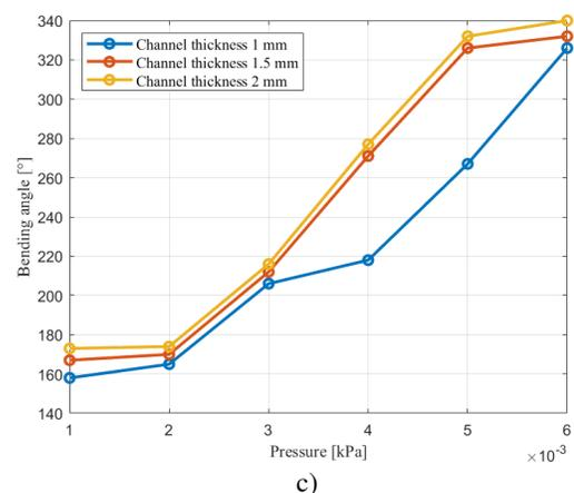
**Fig. 8.** The effect of air channel thickness for: a) the actuator with a rectangular cross-section, b) the actuator with a semi-circular cross-section, c) the actuator with a triangular cross-section.
