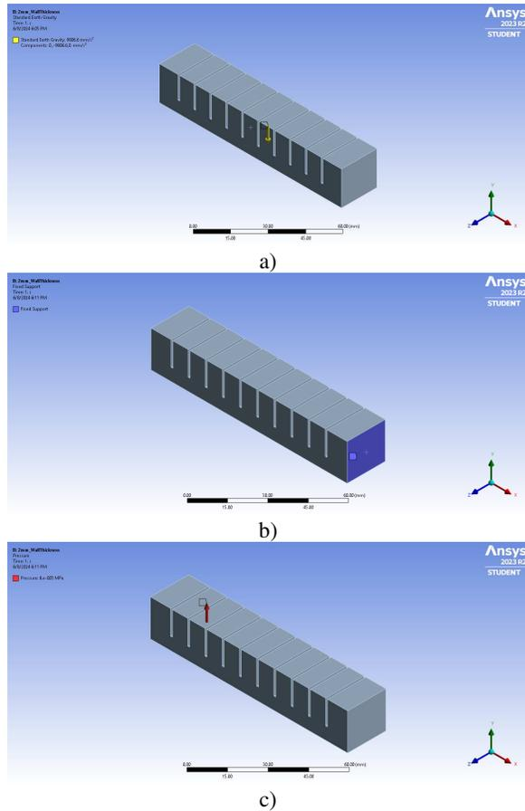
**Fig. 3.** Application of boundary conditions: a) application of gravitational field, b) application of fixed support, c) application of internal pressure.
