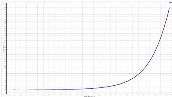
**Fig. 2.** Graph of uniaxial tensile test for Ecoflex 00-50 and second-order Ogden model.
