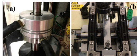
Fig. 3: (a) FMVP and (b) TE-77 shock absorber test configurations.
