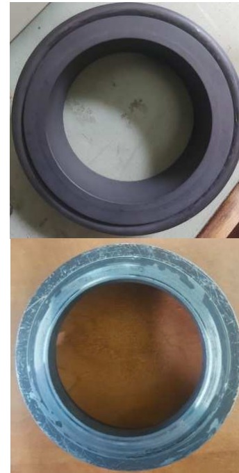
Fig. 12. Faces of the two rings after testing
