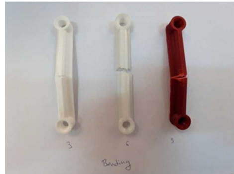
Fig. 7. View of the specimens after the bending tests (Source: Authors).
