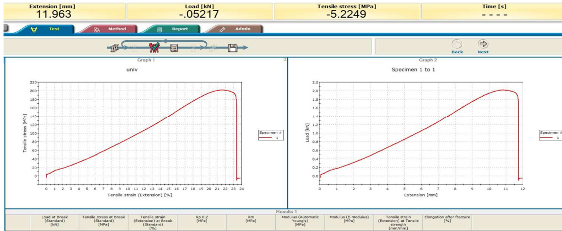
Fig. 14. Graphic representation of sample 7 - ABS filament test results (Source: Authors).
