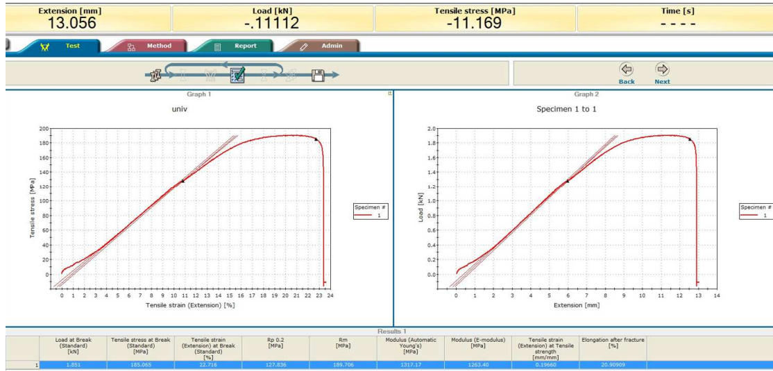
Fig. 10. Tensile curve for a specimen made of PLA filament ( Source: Authors ).
