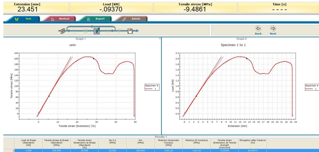
Fig. 12. Graphical representation of sample 4 – filament PC test results (Source: Authors).
