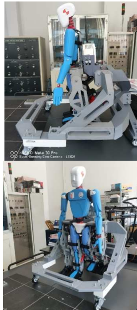
Fig. 9. Exoskeleton prototype with Chebyshev, pantograph and Stephenson III six-bar mechanism for children walking assistance
