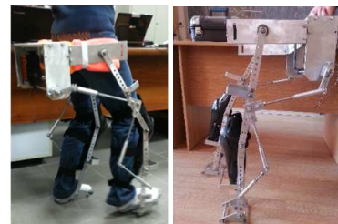
Fig. 5. Exoskeleton prototype without cam mechanism
