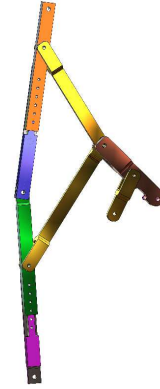
Fig. 3. The 3D model of the exoskeleton leg mechanism.
