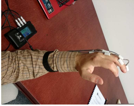
Fig. 2. The goniometer placed on the finger used for data acquisition [14]
