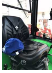
Figure 7. Accelerometers on the driver's seat and cap
