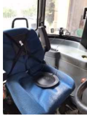
Figure 5. Mounting accelerometers on the seat and seat back
