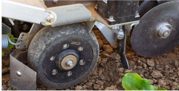
Fig. 7. Precision inter- and intra-row weeding using the FarmDroid FD20[16]
