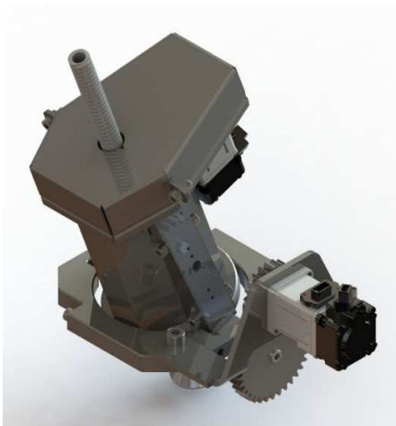
Fig. 4. 3D model of the steam delivery system at the soil surface, in a rotated position
