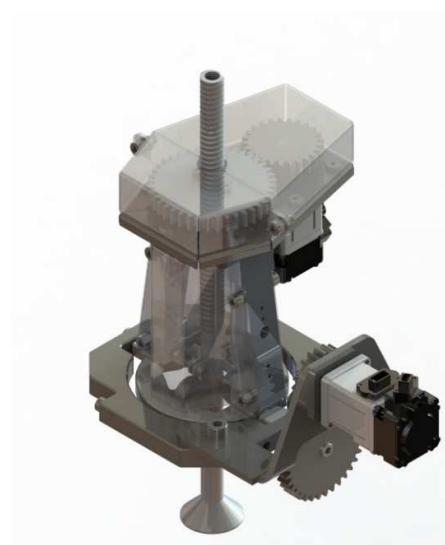
Fig. 1. 3D model of the proposed steam-based weeding module with cover.
