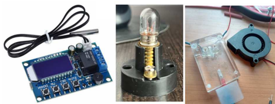
Fig.11. Components used to control the temperature in the room where the measurement takes place
