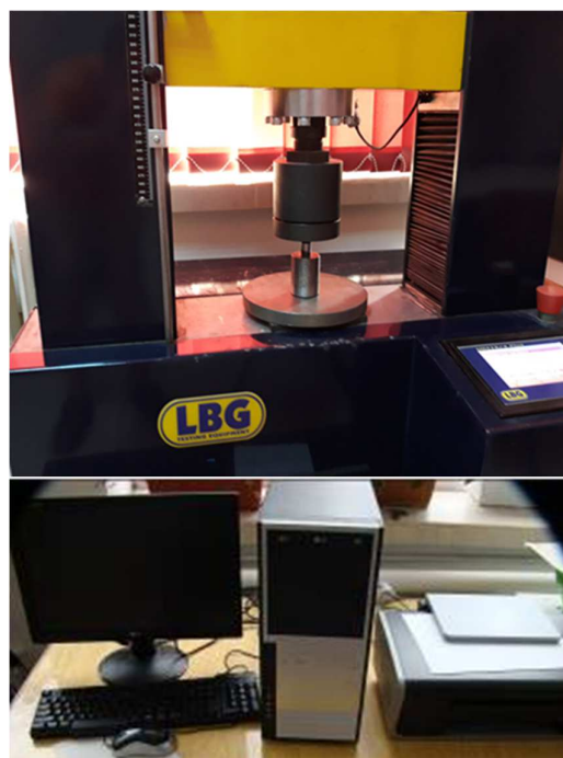
Fig. 2 Compaction equipment LBG Universal Testing Machine
