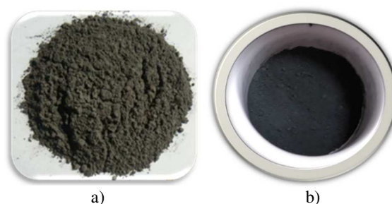
Fig. 1 \text{TiB}_2 powders: a) commercial; b) milled
