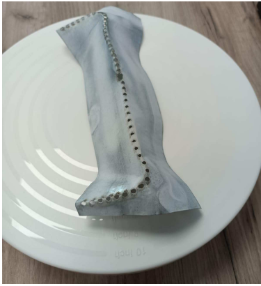
Fig. 9. Scanned piece after applying AESUB orange
