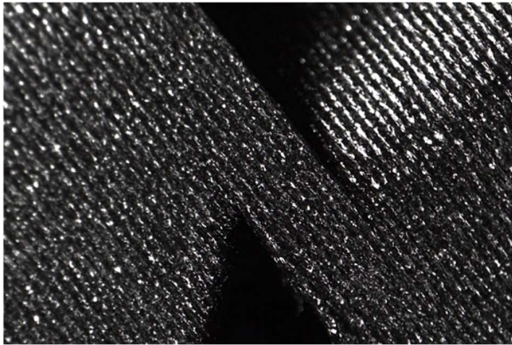
Fig. 7. Picture of the FDM part showing the layer lines
