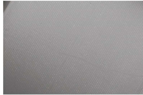
Fig. 9. Image showing the layer lines of the SLA 3D printed part
