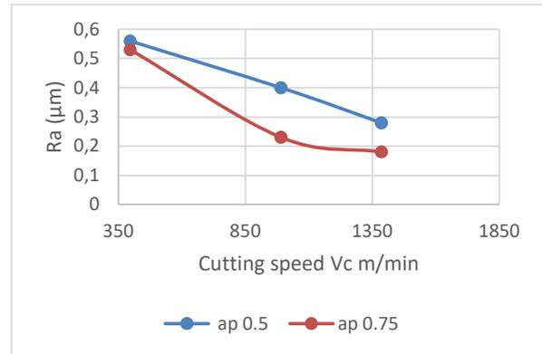
Fig. 3. Influence of cutting speed on surface roughness in dry milling condition.
