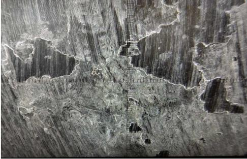
**Fig. 8.** Detailed deposits on the surface 20x measured on Mitutoyo TM101 microscope.
