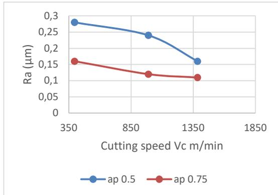
**Fig. 5.** Influence of cutting speed on surface roughness in cryogenic milling conditions.
