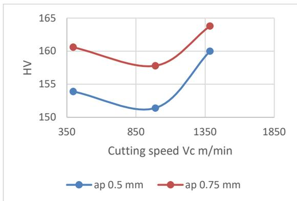
**Fig.6.** Influence of cutting parameter on surface microhardness in cryogenic milling conditions.
