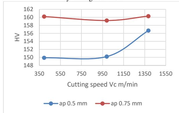
Fig. 4. Influence of cutting parameter on surface microhardness in dry milling condition.
