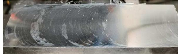
**Fig. 7b.** Cryogenic cooled milled surface (Vc 314 m/min; ap 0.5mm).
