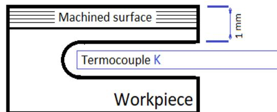
Fig. 2. Thermocouple position in the work piece.
