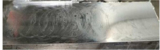
**Fig. 7a.** Dry milling generated surface (Vc 314 m/min; ap 0.5 mm)
