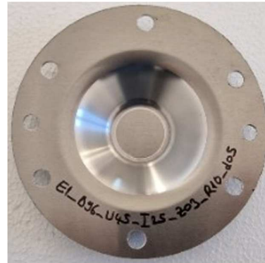
Fig. 12. Image of the part incrementally deformed using a hemispherical head tool with radius R=10 mm.
