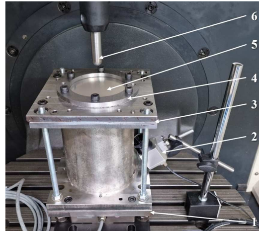
Fig. 4. Experimental stand: 1 - Dynamometer; 2 - Thermographic camera; 3 - Device for orienting and fixing the workpiece; 4 - Workpiece clamping ring; 5 - Workpiece (sheet metal); 6 - Tool.
