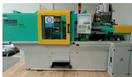
Fig. 2. Arburg 370 S injection molding machine.
