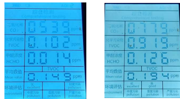
Fig. 9. Emission in the room without the operator left and with operator right.
