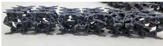
Fig. 10. 3 different structures after the compression test, having the layer thickness in order from left: adaptive, 0.1 mm, 0.05 mm
