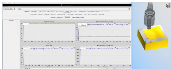
Fig. 4. Analysis of chip thickness, radial and axial forces, power consumption and cutting tool deflection during face milling operation.
