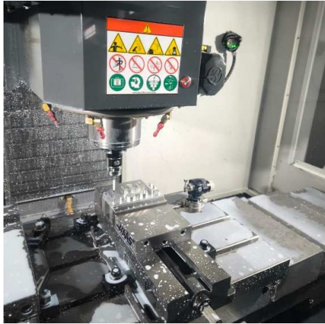
Fig. 3. The Haas Wireless Intuitive Probing System
