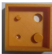
Fig. 6. Prismatic cuboid printed and few geometric and kinematic parameters.
