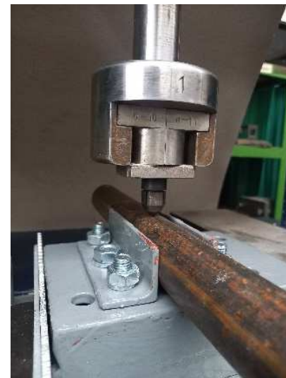
Fig. 10. Fastening the pipe in the clamping device and applying the punch to the pipe.
