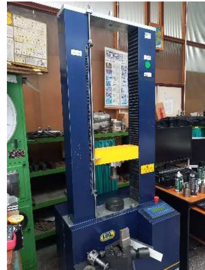
Fig. 9. UDI 16/4 Compression test Machine with soft TCSof2004Plus.
