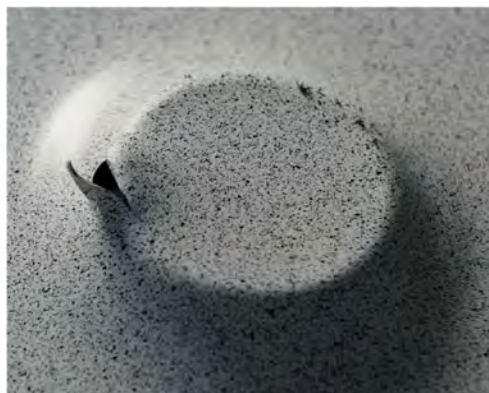
Fig. 4. The unperforated part after the fracture occurs
