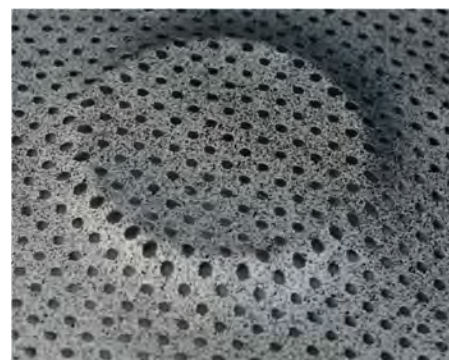
Fig. 8. The perforated part after the fracture occurs
