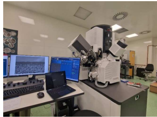
Fig. 2. SEM Microscope Used for the Microstructural Analysis of the Clad Material.
