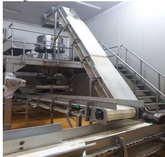
Fig 16. Z Transport Conveyor product implemented in the customer production line
