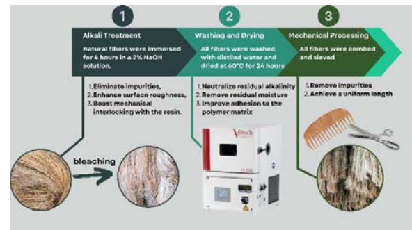
Fig. 1. Effect of Alkali Treatment on Coir Fibers
