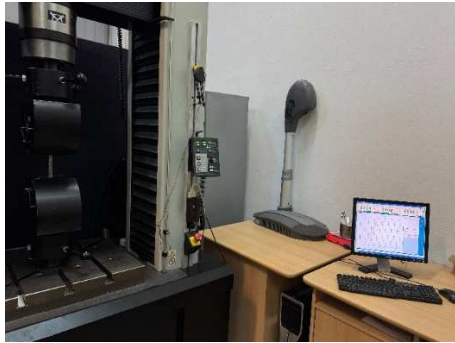
Fig. 4. Uniaxial tensile test on INSTRON 5587.
