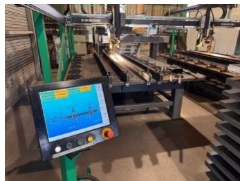
Fig. 3. H-Frame welding machine.
