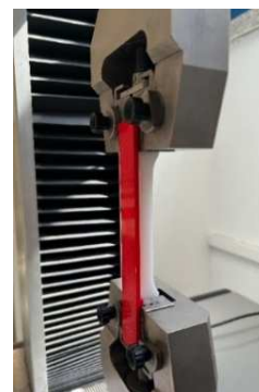
Fig 3. Test specimen attached to the test machine using the device for positioning and orientation
