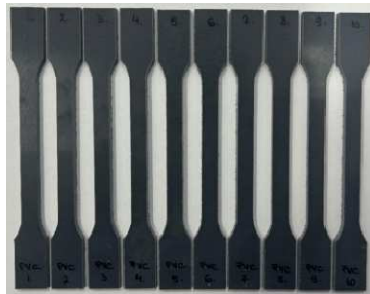
Fig. 5. PVC specimens before tensile tests.
