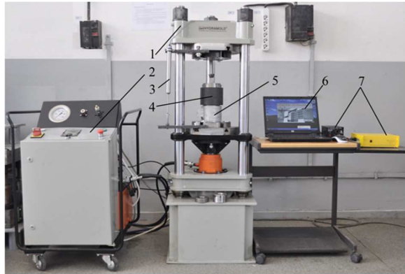
Fig. 1. General view of the deformation force measurement installation: 1 - press; 2 - hydraulic unit; 3 - displacement transducer; 4 - deformation device; 5 - load cell; 6 - notebook; 7 - Traveller 1 system [1]
