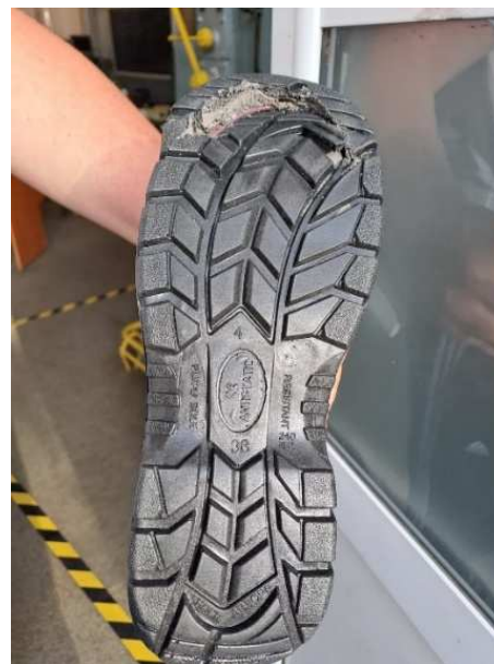
Fig. 5. Severed sole of the shoe after compression test
