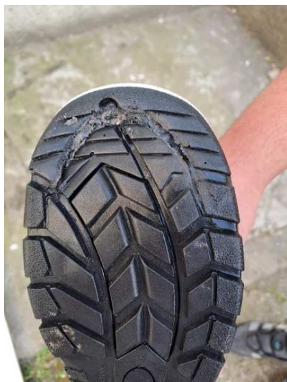
Fig. 12. The sole of the footwear after compression test for 3 min at a force of 15 kN at -36 °C
