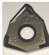
Fig. 5. Image of new cutting-edge 4
