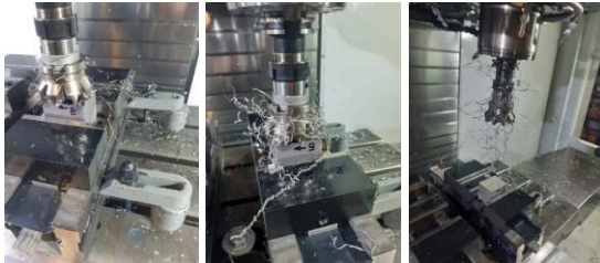
Fig. 14. Change in chip shape
