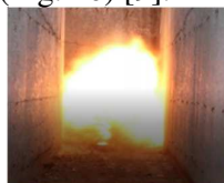
Fig. 9. The explosion resulting from the initiation of the quick-burning fuse, which activated the 190 g of pyrotechnic composition located at the lower part
