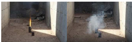
Fig. 3. Triggering / Ceasing the operation of the pyrotechnic article correctly inserted into the metal casing
