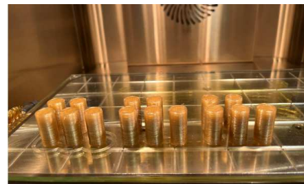
Fig. 2. The compression specimens manufactured with MiniFactory Ultra system.
