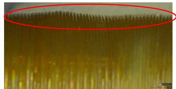
Fig. 14. Local buckling of outer surfaces after compression tests.
