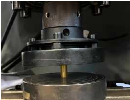
Fig. 5. Compression test for the specimen manufactured using the FFF process.
