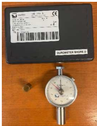
Fig. 6. The Shore D durometer used for the hardness testing of the 3D printed parts.
