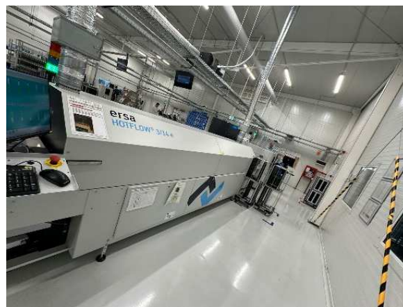
Fig. 9. SMT Reflow Oven with 7 work zones
