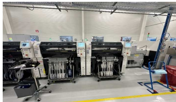
Fig. 8. Automatic Pick and Place Device - Component Feeding Area
