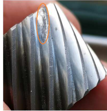
Fig. 14. Fault on the pinion flank
