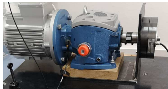
Fig. 1. The test rig: AC motor, VFD, speed reducer, magnetic powder brake
