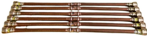
Fig. 3. Crimped specimens with outer diameter D_e = 15 mm and wall thickness w_t = 1.0 mm.
