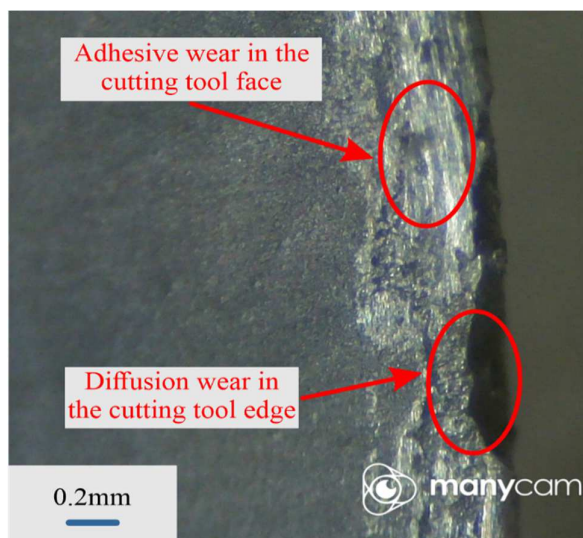
Fig. 12. Adhesion and diffusion zone on the face and cutting edge of a round cutting tool insert
