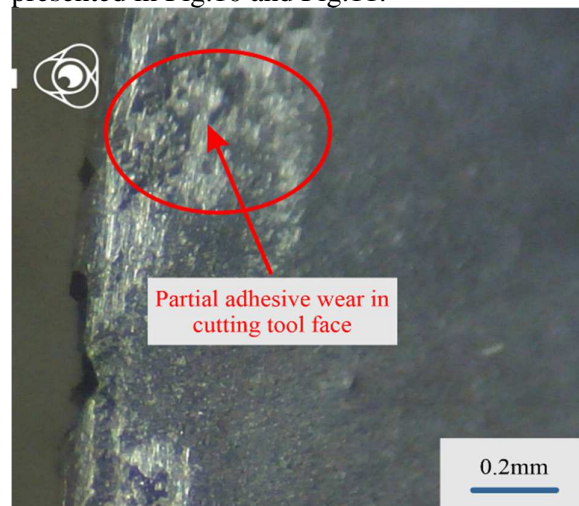
Fig.10. Macro study of the face of a round cutting tool insert (after loading under operating conditions) with observed adhesive wear
