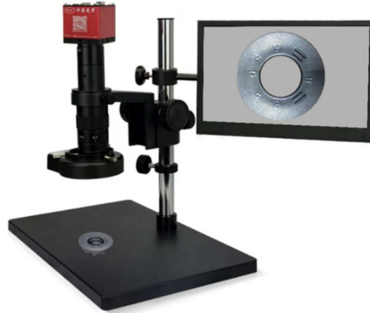
Fig. 6. Digital microscope for wear measurement of round cutting insert
