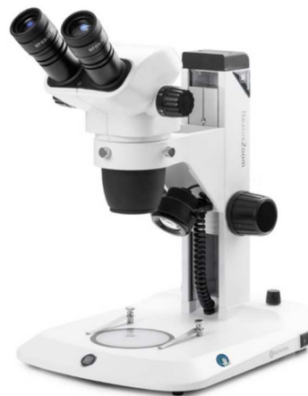
Fig. 7. Binocular stereo microscope for macrostructural studies
