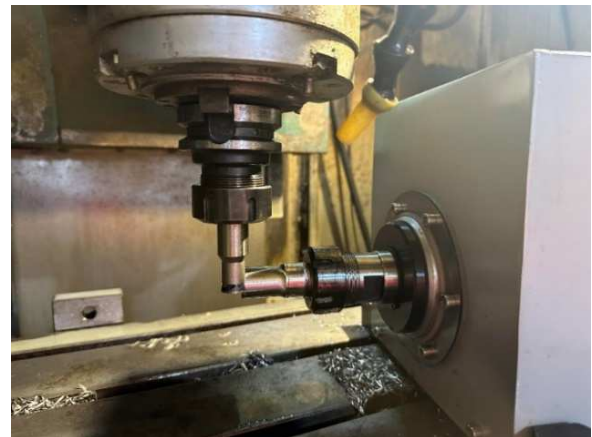
Fig. 4. Machining of a rotation symmetric workpiece with simultaneous rotating tool and workpiece
