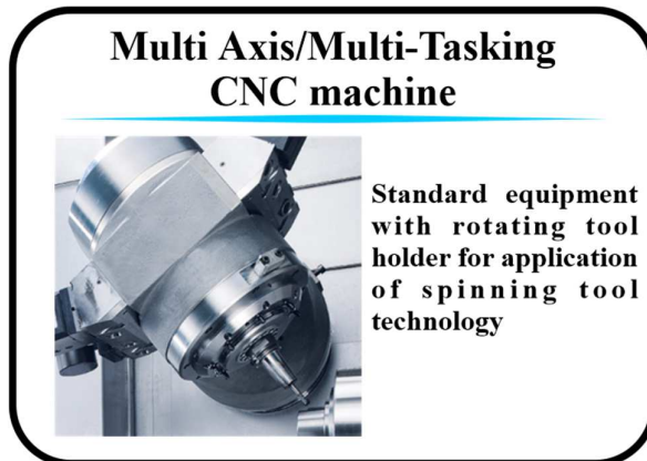
Fig.8. Multi-axis lathe-milling machine equipped with milling spindle
